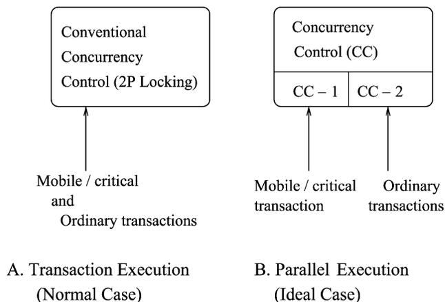
Fig. 2. Transaction management for parallel execution of transactions.
