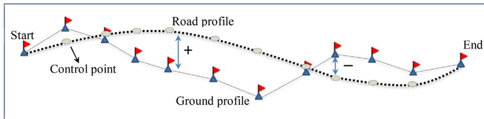
Fig. 1. Side view of ground profile and road profile.
