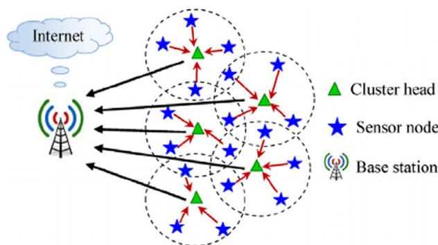
Fig. 1. Typical clustering environment of wireless sensor network.
