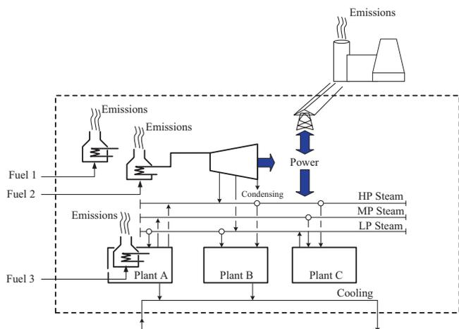
Fig. 1. Typical configuration of an industrial Total Site (after Klemeš et al., 1997).
