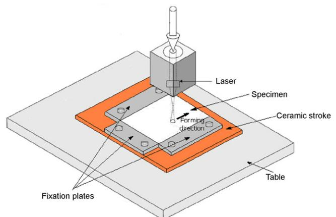
**Fig. 1 – Overview of Laser Beam Forming experimental set-up.**
