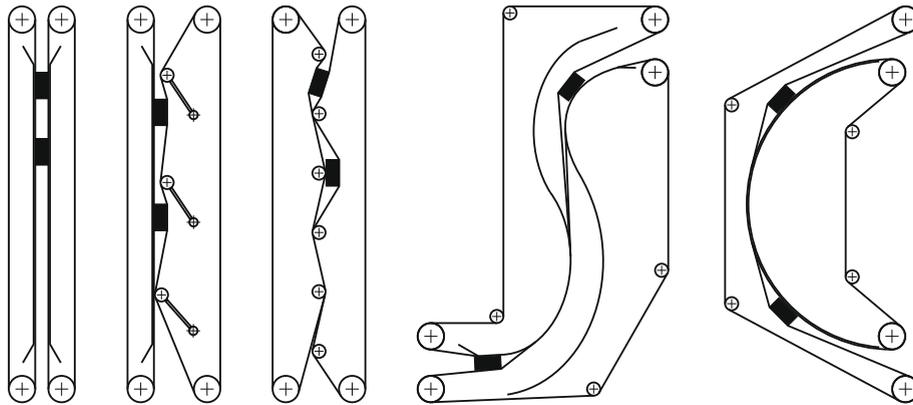
**Fig. 1.** Overview of different design concepts for standard cover belt systems (cp. [6], p. 23, [1,9]). From left to right, the characteristic of the conveying trajectory changes from straight to alternately radial to radial.
