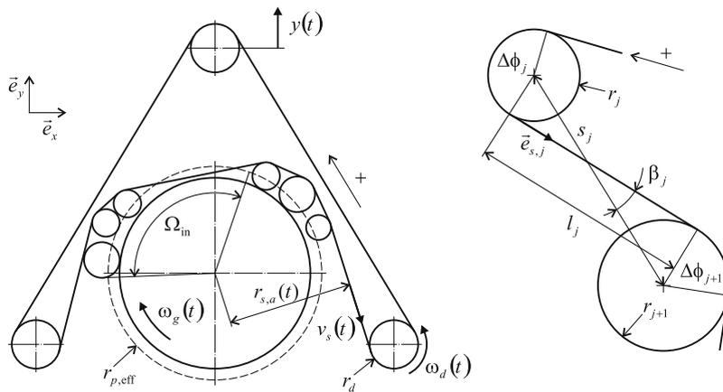
**Fig. 2.** Two-dimensional representation of the cover band system. The left figure shows an exemplary arrangement of pulleys and the basic kinematic factors. The arbitrarily chosen two-pulley arrangement on the right explains further basic parameters used for the geometric modeling.
