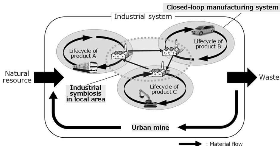
Fig. 1. Existing concepts of resource-circulating manufacturing systems.
