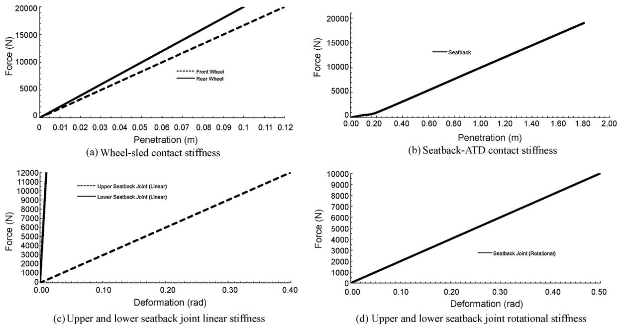
**Fig. 1.** Key computer model stiffness characteristics. (a) Wheel-sled contact stiffness; (b) seatback-ATD contact stiffness; (c) upper and lower-seatback joint linear stiffness; (d) upper and lower-seatback joint rotational stiffness.
