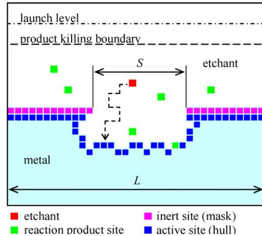
Fig. 1. 2D etching simulation model.
