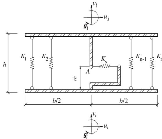
Fig.1 Multi-Vertical-Line-Element Model
