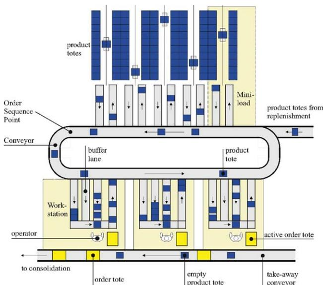
Fig. 1. Miniloading-workstation order picking system.
