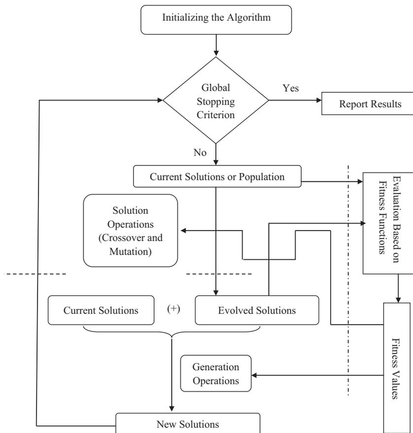
Fig. 1. Basic evolutionary operations of evolutionary algorithms.
