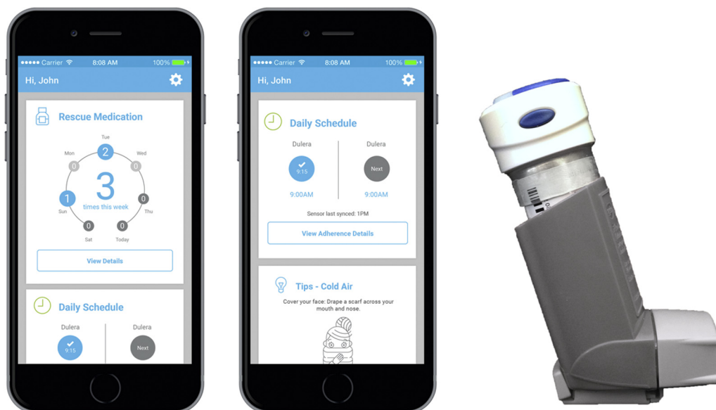
Figure 1. Electronic sensor attached to a metered-dose inhaler canister, paired with the smartphone and web applications that present visualized data and trends.
