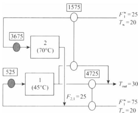
Figure 2 Solution for Example 1 not allowing operation split
