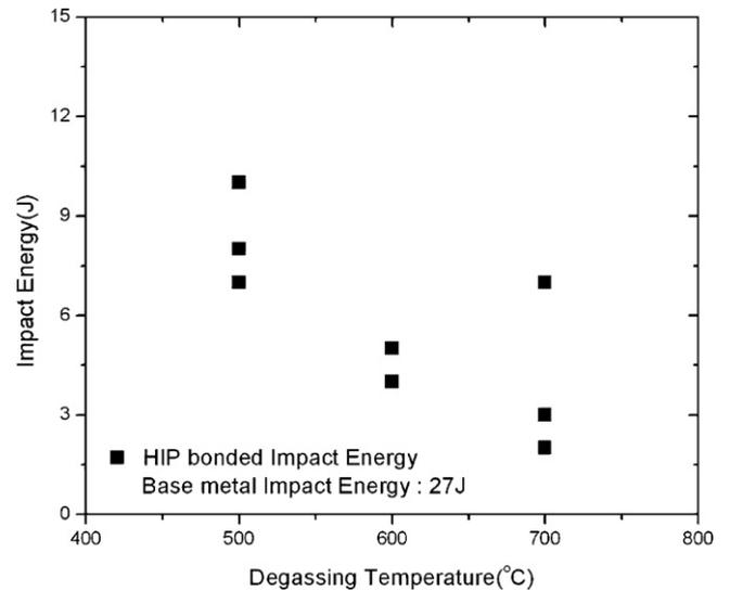
Fig. 2. Charpy impact energy of HIP bonded specimens.
