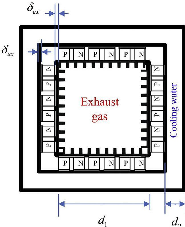
Fig. 1. Schematic diagram of the heat transfer passage cross section.
