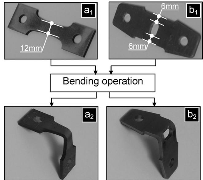
Fig. 1. Initial (a<sub>1</sub> and b<sub>1</sub>) and final (a<sub>2</sub> and b<sub>2</sub>) steps of bending tests.
