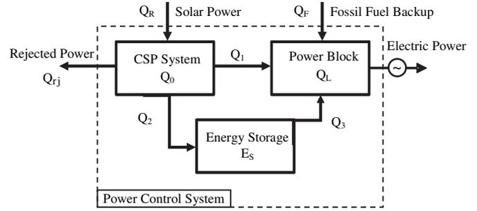
Fig. 1. The schematic model of a solar thermal electric power system.
