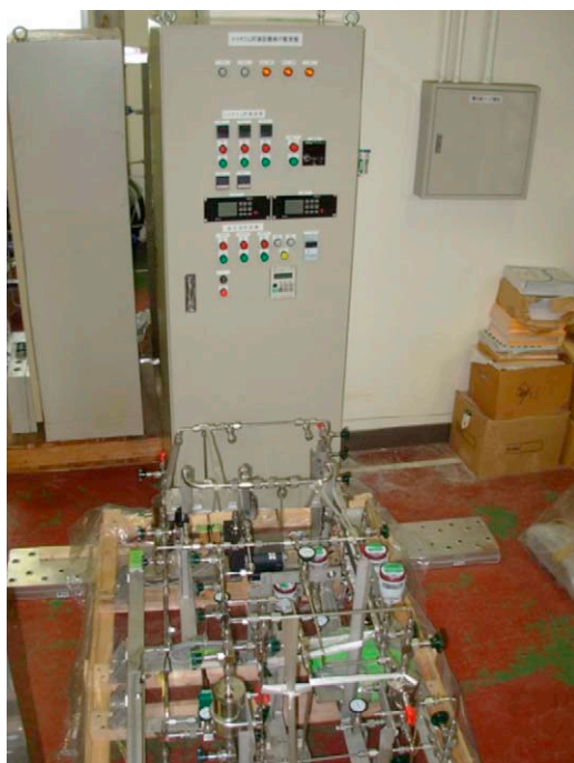
Fig. 1. Photograph of tritium storage bed ( 7.4\text{ TBq} ) using ZrCo powder at Rokkasho.
