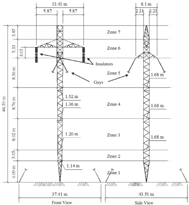
Fig. 1. Schematic of the full-scale guyed transmission tower.
