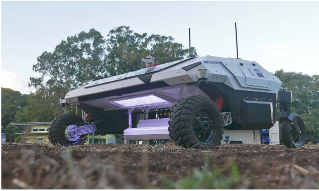
Fig. 1. AgBot II agricultural robotics platform.
