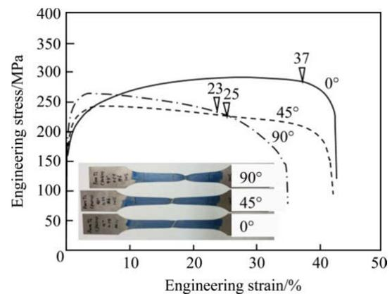
**Fig. 3** Engineering stress–engineering strain curves of titanium sheet obtained from tensile tests
