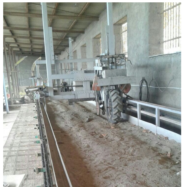
Fig. 1. The general testing of soil bin facility and single-wheel tester for conducting experiments.
