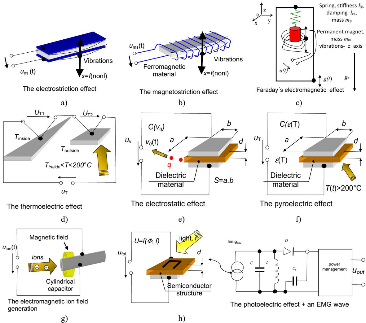
**Fig. 1.** The principles of energy harvesting: (a) the electrostriction effect; (b) the magnetostriction effect; (c) Faraday's electromagnetic effect; (d) the thermoelectric effect; (e) the electrostatic effect; (f) the pyroelectric effect; (g) the generation of a moving electromagnetic ion field (EMHD generator); (h) the photoelectric effect and an EMG wave harvester [13].
