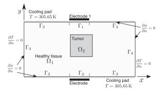
**Fig. 1.** A simplified 2D model of a radiofrequency induced thermal treatment (hyperthermia) with an embedded tumor.
