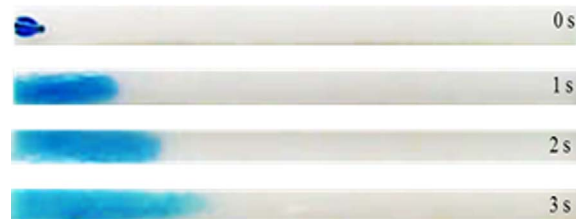
Fig. 4. A set of time series photos showing increasing migration distance after adding 10 \mu l dye solution on the noodle platform II.
