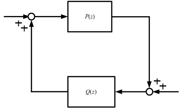
Fig. 1. Positive feedback interconnection of  $P(z)$  and  $Q(z)$ .
