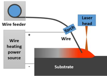
Fig. 1. Schematic of laser hot-wire deposition
