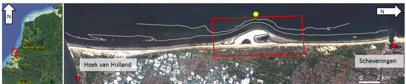
Fig. 1. Overview of the Dutch Delfland coastal cell bordered by Hoek van Holland (left) and Scheveningen (right). The Sand Motor study site is indicated in red. Depths at the -8 m, -5 m and +2 m NAP iso-contours are indicated in grey. The underlying satellite image (SPOT mission) was acquired on 18-05-2014. The water level measurement stations of Hoek van Holland and Scheveningen are indicated by means of a red dot. A nearshore location at the -10 m NAP depth contour, on which nearshore wave data are available, is indicated in yellow. (For interpretation of the references to colour in this figure legend, the reader is referred to the Web version of this article.)
