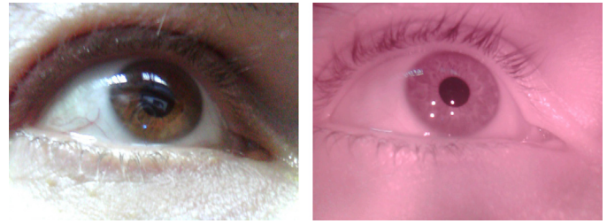
Fig. 2. The same eye image recorded by the same digital camera with and without IR filter (Genius FaceCam 2025 with IR filter switch). It is visible that a pupil is much easier to find on the infra-red image.
