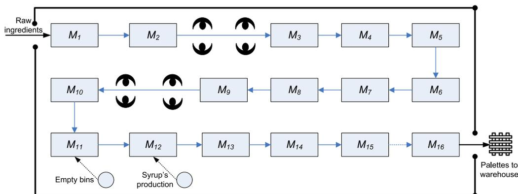
Fig. 1. Schematic presentation of peach production line.
