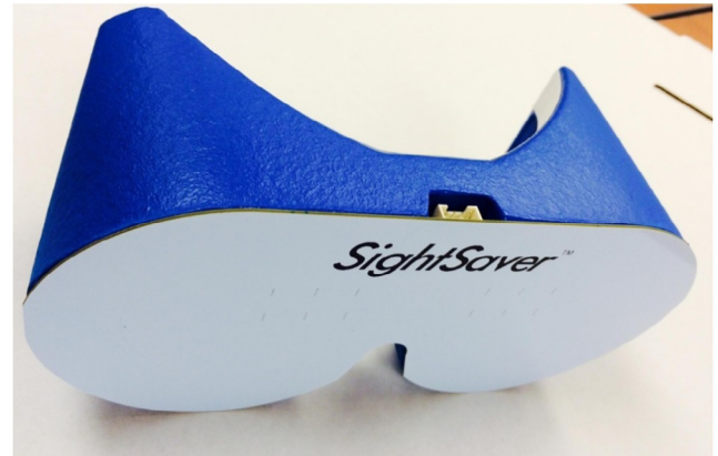
Fig. 1. The SightSaver™ flash visual evoked potential stimulator.
