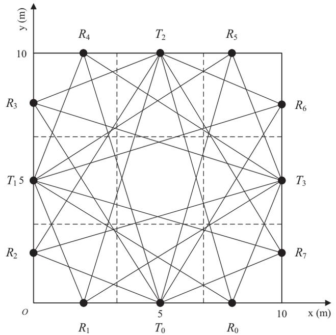
Fig. 1. A typical ultrasonic transmitter and receiver layout installed in a measurement region.
