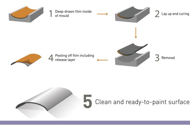
Flex<sup>PLAS®</sup> is deep-drawn into the mold like a second skin in place of the release agents typically used in composite manufacturing. Highly elastic and thermally stable at up to 190°C, Flex<sup>PLAS®</sup> can be used in many equipment types and processes.
