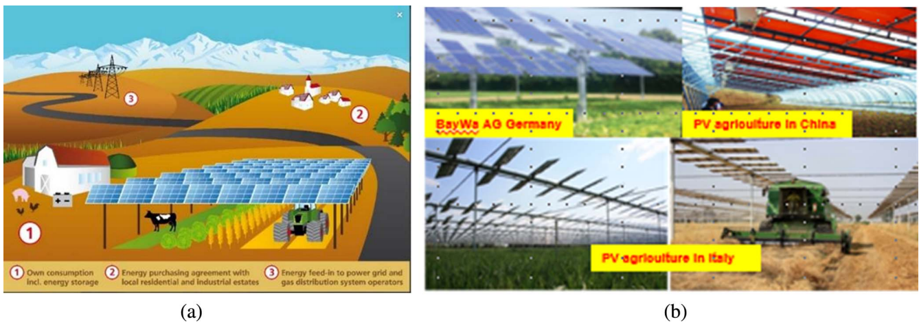
Fig. 1. (a) The basic principles of agriculture photovoltaic; (b) current solution for agriculture photovoltaic by implementing mosaic type of solar panels structures high above the farmland.
