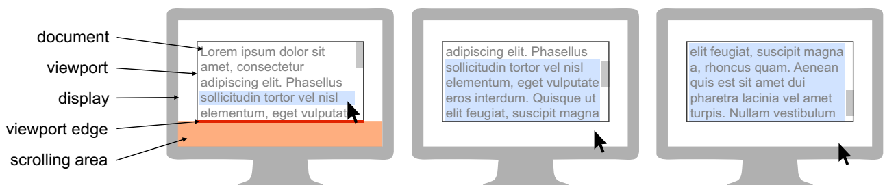
Fig. 2. Edge-scrolling is used in the course of a task (here, selecting text) in order to scroll a document that is displayed inside a viewport placed on the display . The user activates edge-scrolling by entering a scrolling area near the viewport edge (left). Inside the scrolling area, pointing actions control the pace of scrolling (middle, right).
