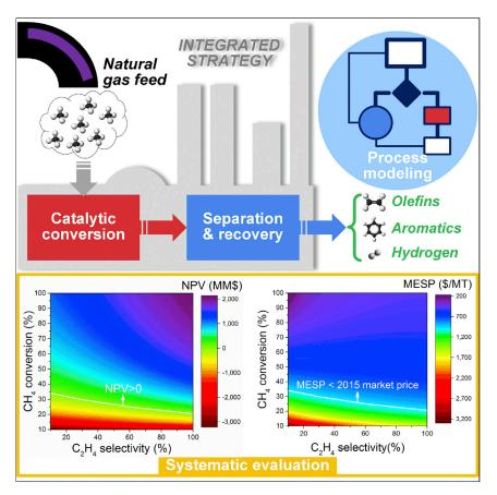
Natural gas is a versatile chemical feedstock. While the direct conversion of methane to olefins and higher hydrocarbons has received significant attention, there exist a number of open questions regarding the development of cost-effective methane-to-chemicals integrated processes. To address some of these questions, we develop a general systems-level framework for the systematic evaluation of various strategies and the identification of key technology gaps and economic drivers.
