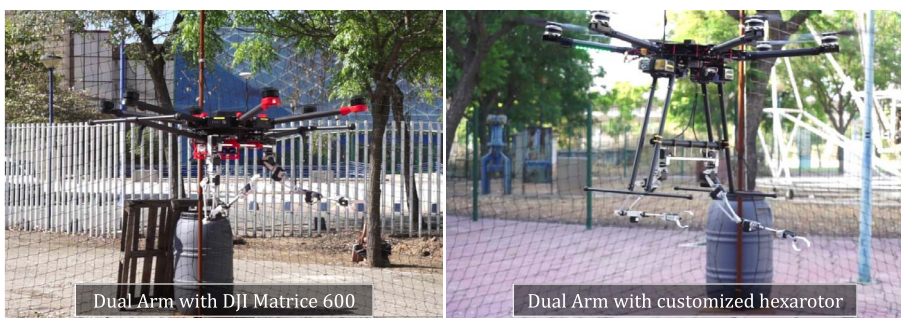
Fig. 1. Developed lightweight and human-size dual arm manipulator integrated in two hexarotor platforms. Outdoor flight tests.
