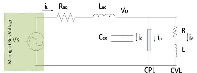
Fig. 4. Equivalent circuit of AC microgrid with CPL & CVL [14].
