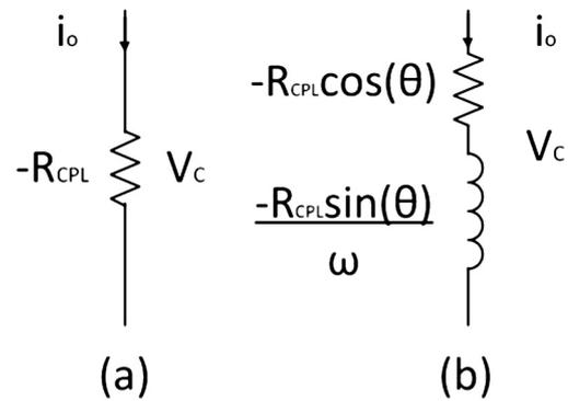
Fig. 2. Small signal representation of a CPL (a) with unity power factor regulation (b) and with lagging power factor [7].
