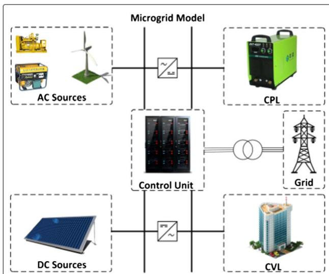
Fig. 1. Typical model of grid-connected microgrid with different distributed generations and loads.
