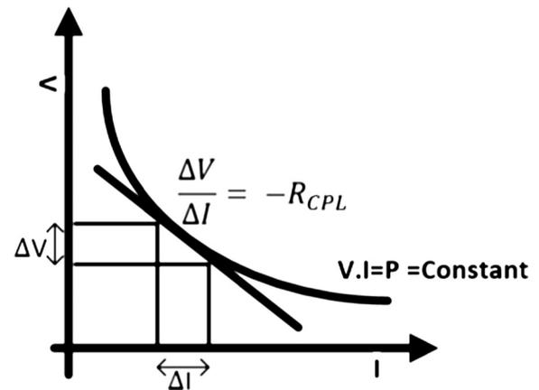
Fig. 3. Negative impedance characteristic of CPL [16].
