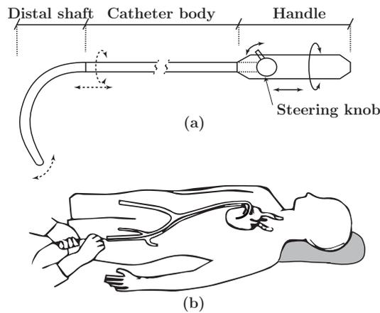
Fig. 1. Schematic view of a steerable catheter (a). Manual catheterization (b).
