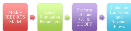
Fig. 1. Simulation methodology: after careful selection of IEEE RTS model and simulation parameters, a 24-h Day Ahead (DA) unit commitment and dispatch is performed, and the resulting emissions and revenue flows are calculated.
