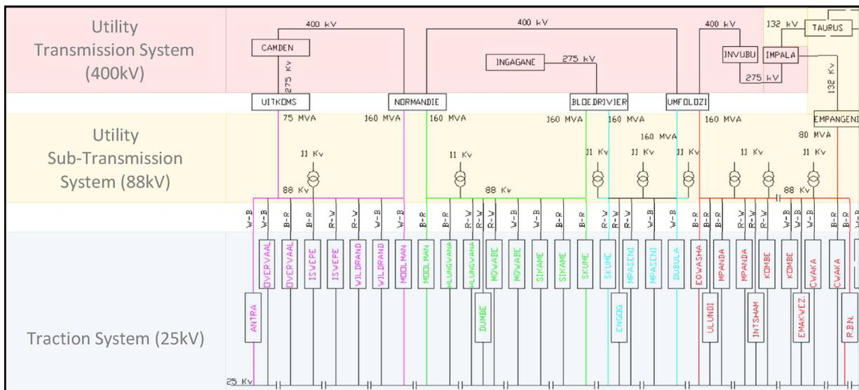
Fig. 1. Single line diagram of the traction and utility network interface [3]. (For interpretation of the references to colour in the text, the reader is referred to the web version of this article.)
