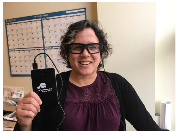
Fig. 1. Eyewear-embedded camera. Eyewear-embedded camera was used to capture still images at the rate of 2 shots/min throughout the course of one day. A pocket-sized external battery was connected to the camera, which was carried on or near the participant's person.
