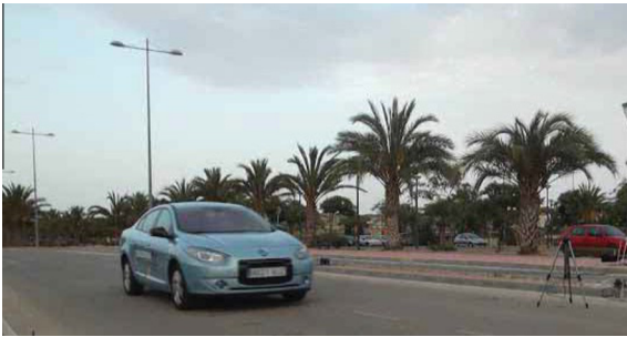
Fig. 1. Pass-by test of an electric vehicle.
