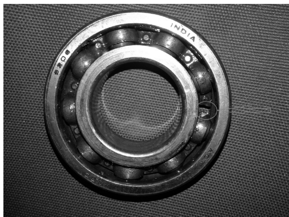
Fig. 2. Bearing with cage fault.
