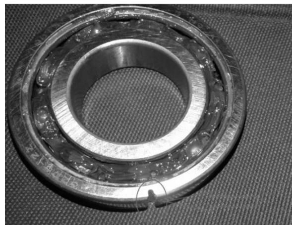
Fig. 3. Bearing with outer race fault.
