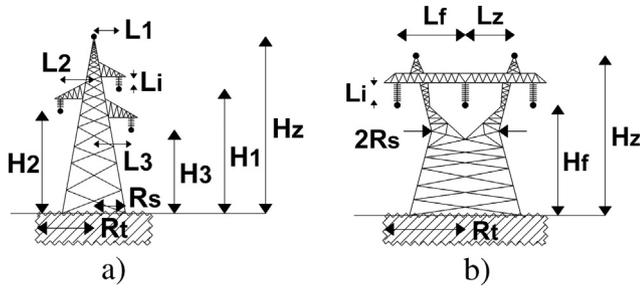
Fig. 1. Overhead lines towers configurations: (a) 35 kV, 110 kV and (b) 220 kV.
