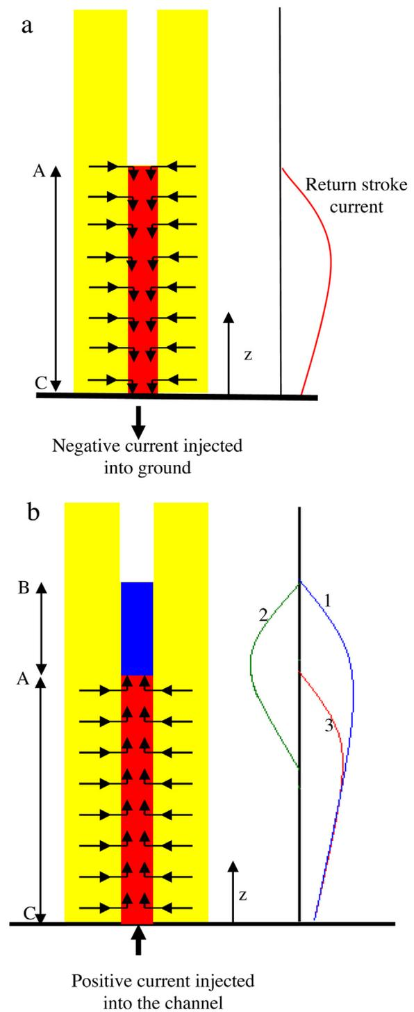
**Fig. 1.** (a) Pictorial description of the current generation (CG) concept. According to CG concept the downward moving corona currents generate the return stroke current. Adapted from Ref. [11]. (b) Pictorial description of the current dissipation concept. Waveforms to the right depict different current components along the channel. (1) Injected current. (2) Upward moving corona current. (3) Net current along the channel. (Adapted from Ref. [9]).
