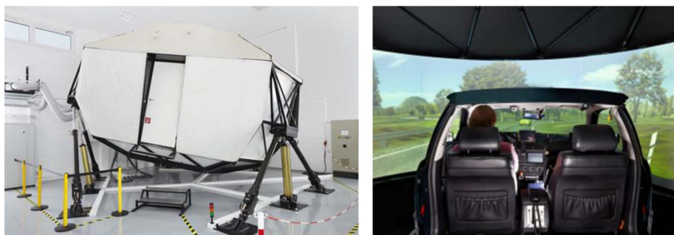
Fig. 1. The WIVW moving-based driving simulator. Hexapod movement system (left) and simulator interior with vehicle mock-up and image projection (right).
