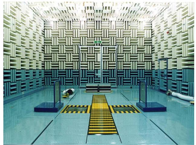
Fig. 1. Semi-anechoic room and dynamometer for sound recording.
