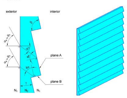
Fig. 1. Geometry of frontal asymmetrical prism.
